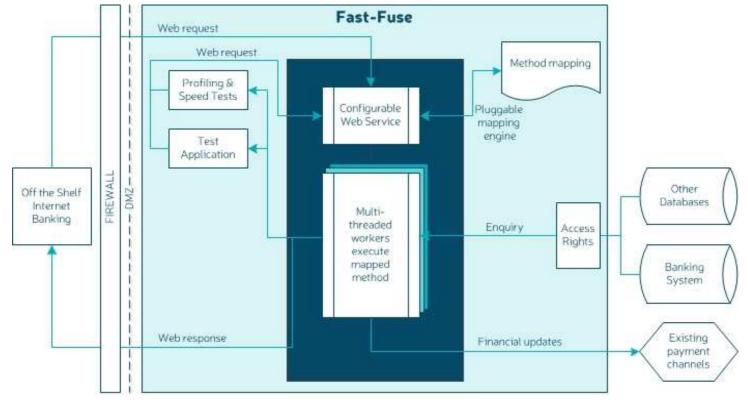
Fast-Fuse is a set of interfacing tools and utilities that facilitates integration between internet banking systems and core banking systems, like BankMaster/BM+. This allows the interaction between newer internet technologies and older core banking technologies without the requirement of replacing the core banking system.
